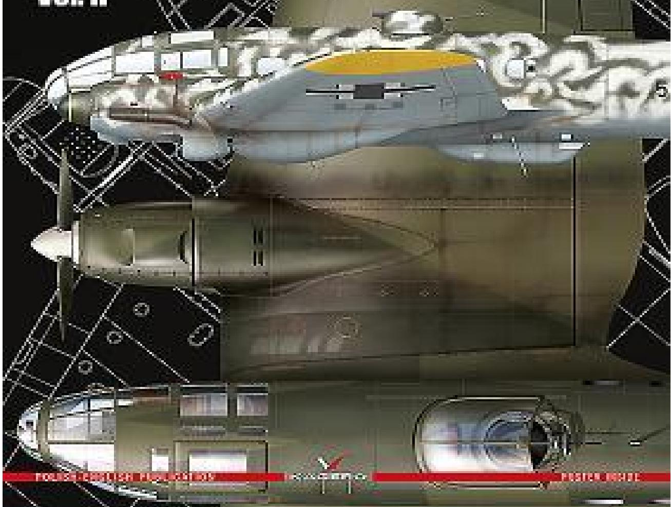
The "H" version of He 111 was the most popular variant of described bomber. The first model of this version - H-0 - was based on the serial He 111P-2 but had Junkers 211A-1 engines, which later were used as a standard propulsion of He 111H variants, eventually replacing lighter, but weaker and difficult to acquire Daimler Benz engines DB 601 units (they were prioritized to fighters).
